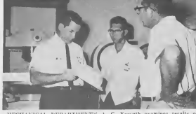
MECHANICAL DEPARTMENT'S A. G. KOSBUTH examines results of crushing test on newly purchased safety hats while A. Vrolijk and J. Abraham look on. Hats withstood 3100 pounds of pressure.
